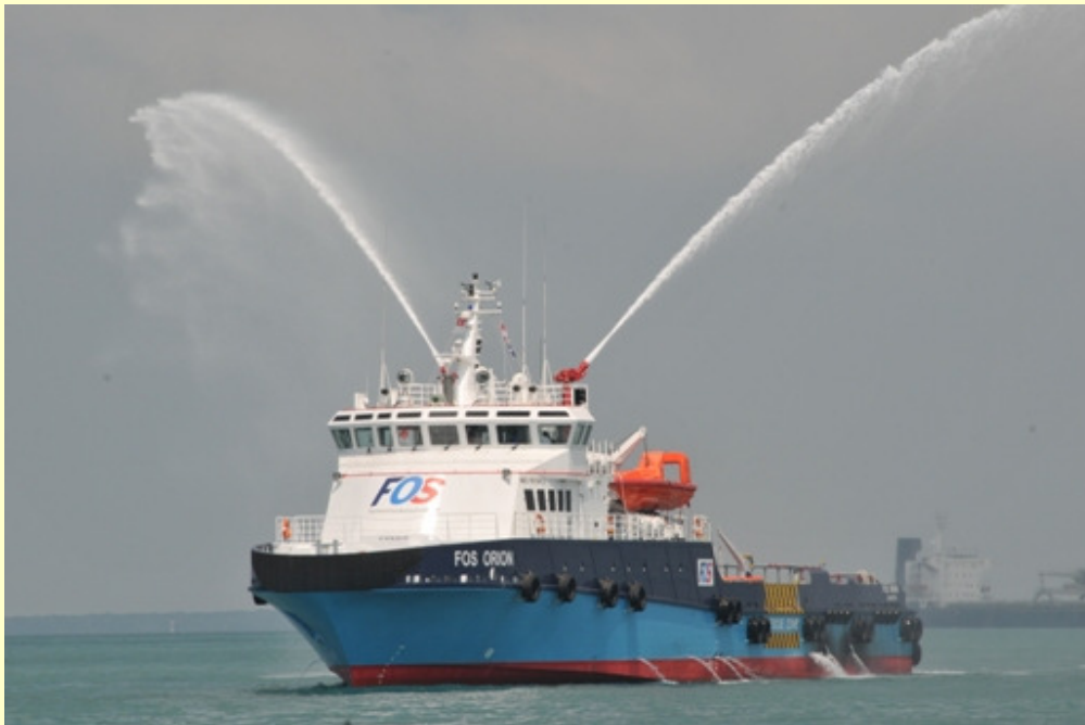
Fire Fighter "FOS Orion" powered by Cat engine models 3516 and C9, all set to play her role in supporting the oil companies' regional exploration activities.
