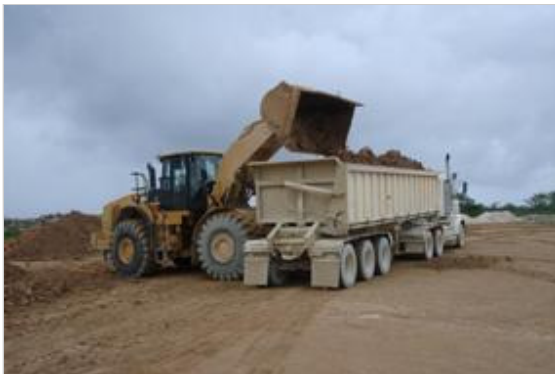
Cat 980H wheel loader, loading from stockpile onto a Kenworth truck, powered by Cat engines.
